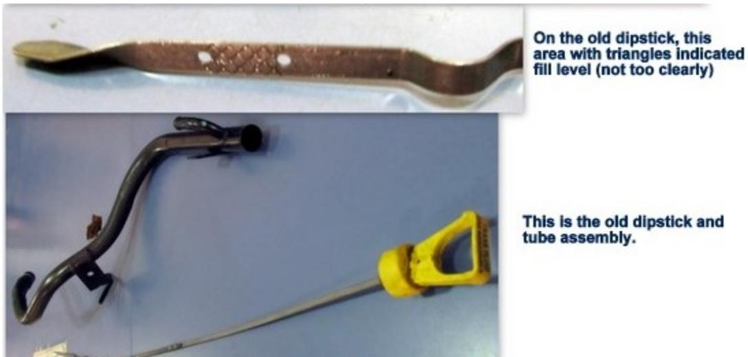
He also installed the new dipstick, and it was only then that I realized it was a bigger deal than just a new dipstick, but included a newly redesigned tube assembly.
